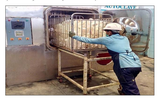
**Fig: Showing Feeding of Waste in the Autoclave Chamber**
